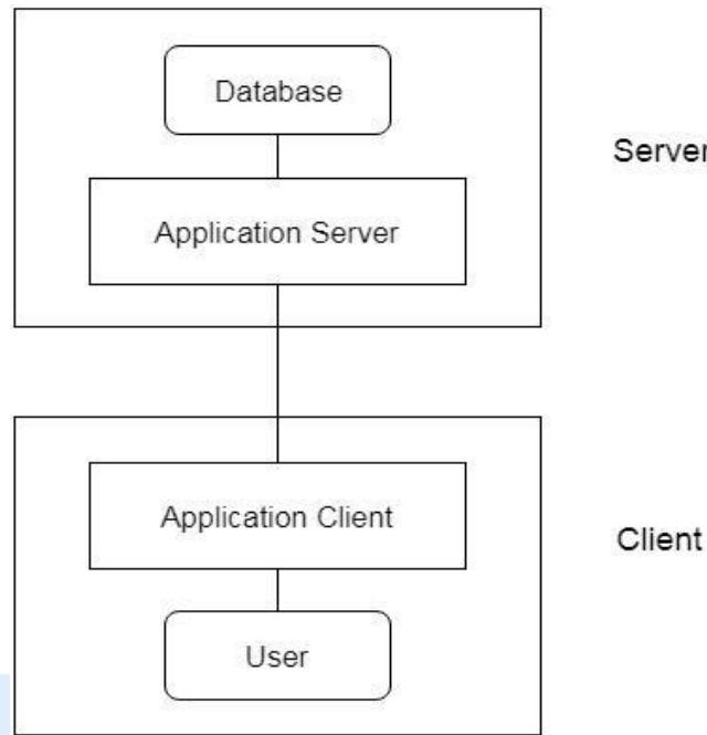
The application on the client-end interacts with an application server which further communicates with the database system.
